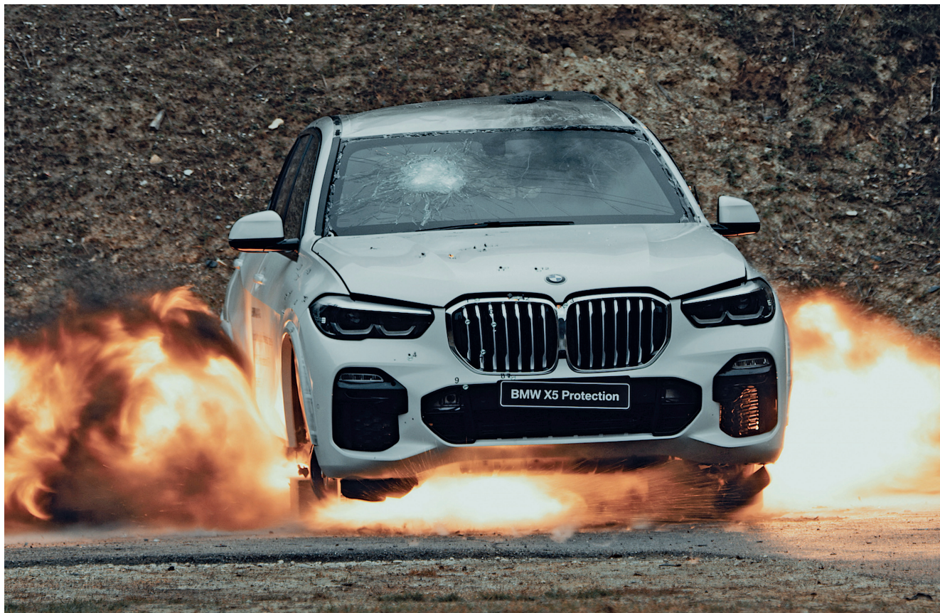
Ballistic panels are being used as armor for civilian and military vehicles, ships and aircraft. The image shows a test blast to demonstrate the safety for vehicle occupants. ©TDW Schrobenhausen
